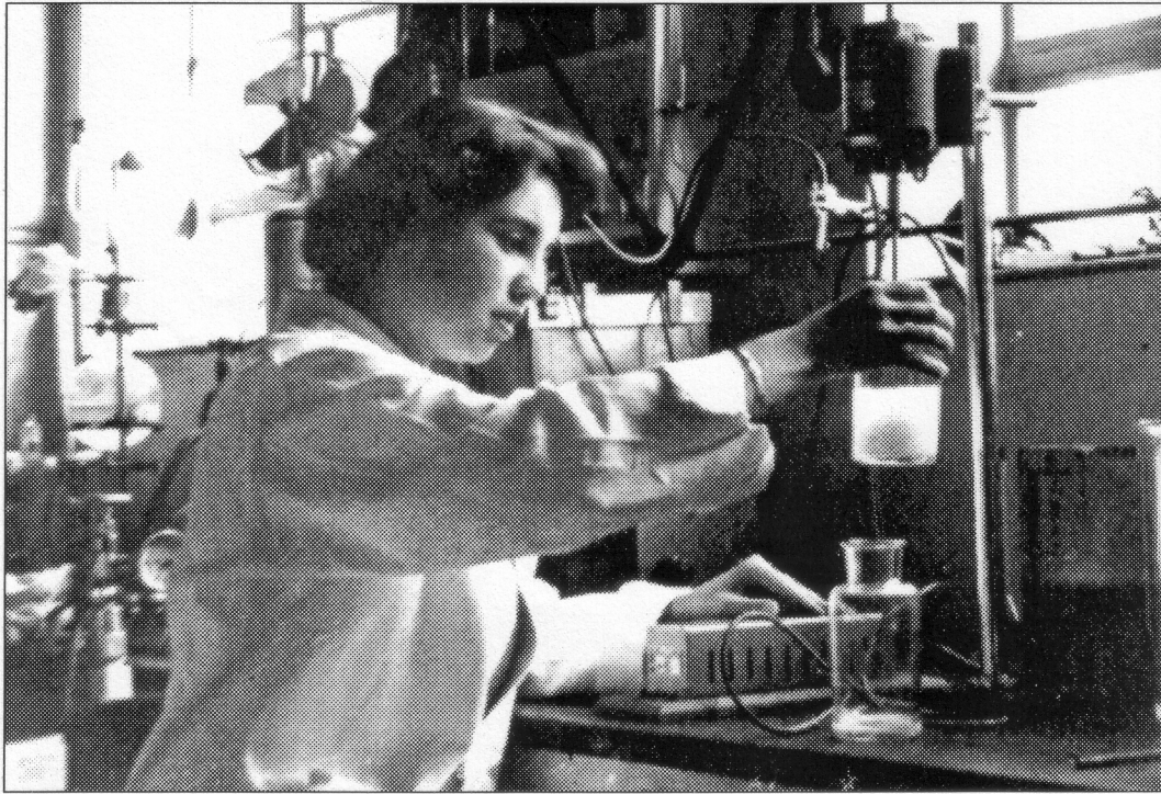
5. The purification is carried a stage further by another precipitation, with sodium citrate.
